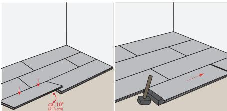
**FIRST ROW:** Start laying in a right corner of the room. Lay the first plank so that the tongue side faces the wall. Align it exactly with spacer wedges. Place the second plank just in front of the first plank and tap it together using a tapping block and hammer. Make sure that the planks are aligned.
