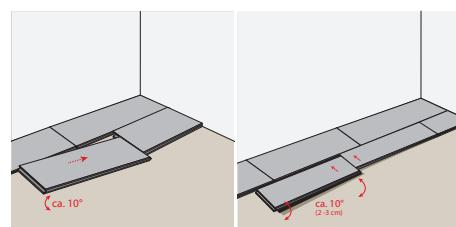
**FIRST ROW:** Start laying in a right corner of the room. Lay the first plank so that the tongue side faces the wall. Align it exactly with spacer wedges. Lever the second plank with its front tongue in exact extension into the front groove of the first plank.
